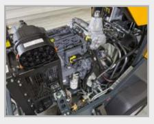
The robust, compact 3-cylinder Deutz engine meets all requirements of the "Stage V" emissions standard, applicable in the EU and Switzerland.
